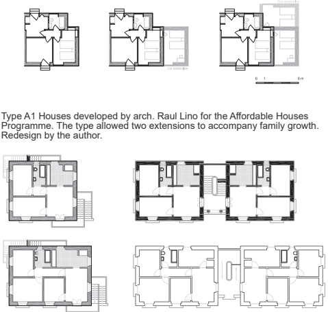
Alvito Affordable Houses Estate House Types. Architect Paulino Montez, Lisbon 1936-44. The same types are used in two-story buildings with independent access (Left) and three-story buildings with common access (Right). Redesign by MdH - Mapping Public Housing Research Project.
