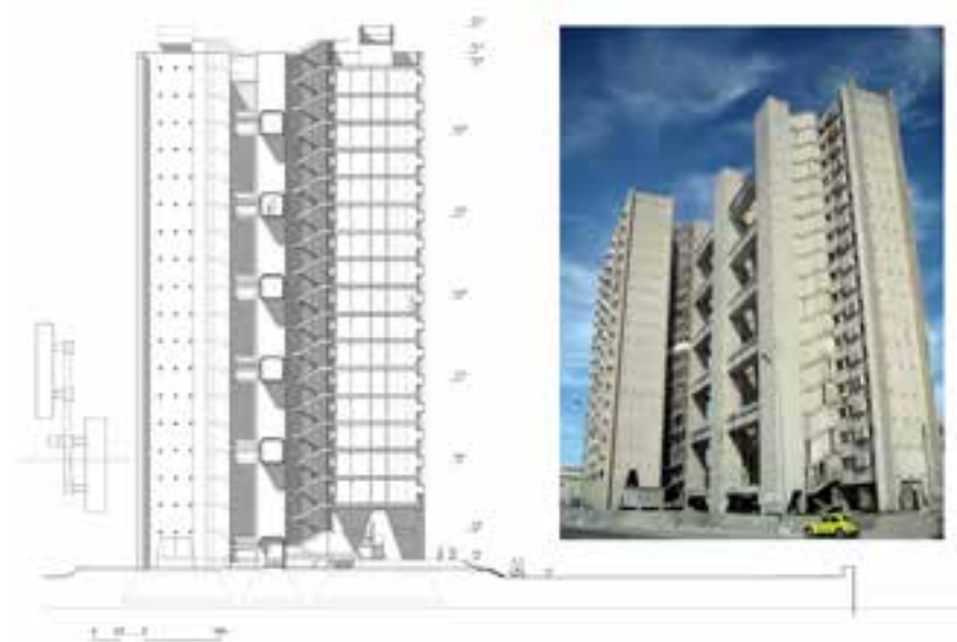
Figure 4. Antonio Quintana and Alberto Rodríguez. Apartment building at Malecón and F (Girón Building) . Havana, Cuba, 1967. Cross-section facing west (4a, left); view of the building from northwest Malecón (4b, right). Produced by the authors based on measurements on site. © Óscar Pedrós Fernández, 2018.
