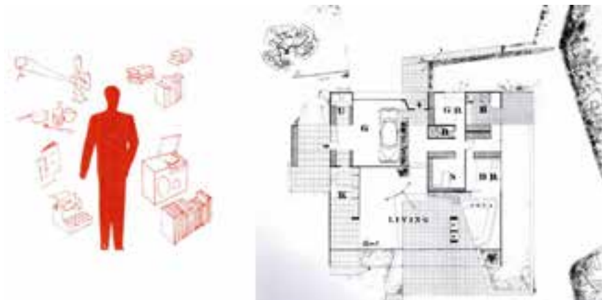
Figure 3. Eames & Saarinen, Entenza House in Pacific Palisades. Left: drawing explaining the editor's interests and requirements for his CSH#9 ( Arts & Architecture , December 1945). Right: plan of the built house ( Arts & Architecture , July 1950).
