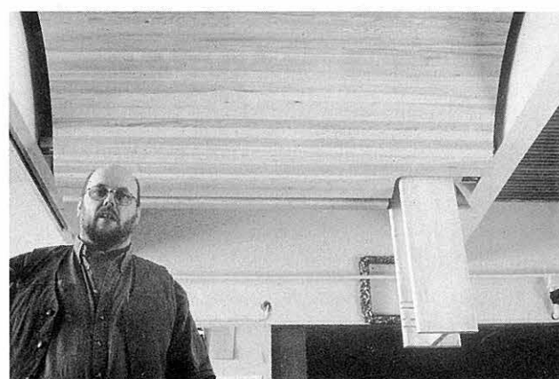
Fig 15. The prototype was mounted in to the intermediate floor in the Heinola Institute. The column was also simulated with a wooden one. Photo M. Heikinheimo.
