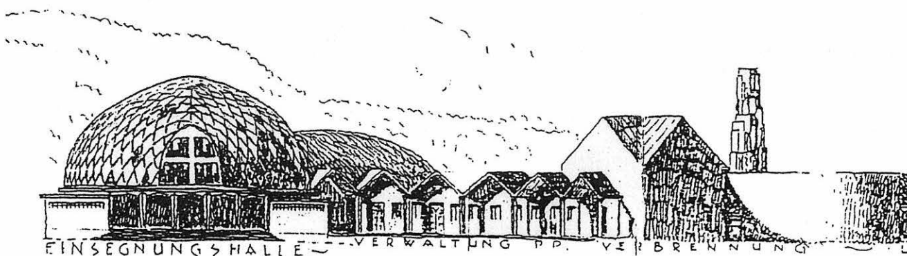
Fig. 27. Design of a confirmation hall for the cemetery South-East in Magdeburg by Bruno Taut, 1922. The Zollinger roof was supposed to cover an oval and circular ground plan.
