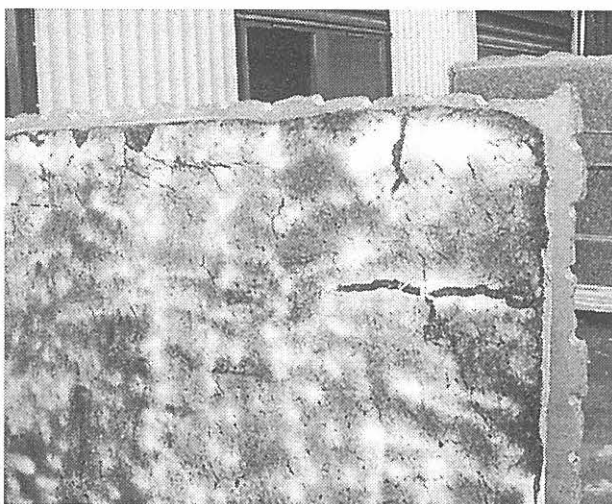
Cracking in granite, due to blast damage during quarrying. Note dye penetration treatment has been used to highlight cracks.
